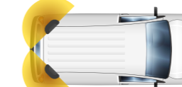
Cat 'HT' Class I 270° wide angle light spread from two units mounted on corners of vehicle
