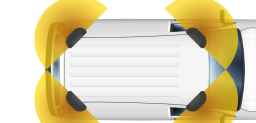
Cat 'T' Class II 360° full-coverage light spread from four units mounted on corners of vehicle
